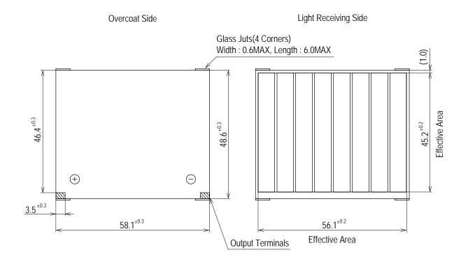
Note: Glass Substrate Thickness : 1.1mm Module Thickness : 1.3mm max Accepts normal soldering for bending.
