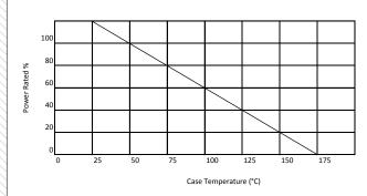
The case temperature is to be used for the definition of the applied power limit
