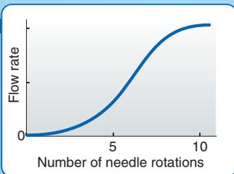
Numerical indication of handle rotation for flow rate reduces flow setting time and setting errors!
