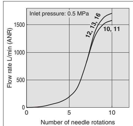
Note) The numbers above the flow-rate characteristic curves in the charts show the applicable tubing outside diameter as defined by the product number.
