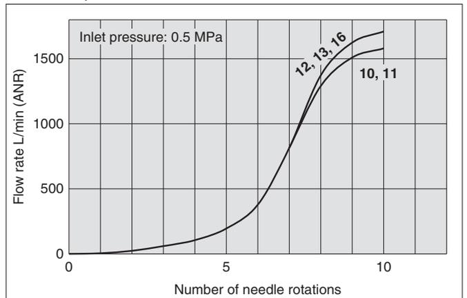
Note) The numbers above the flow-rate characteristic curves in the charts show the applicable tubing outside diameter as defined by the product number.
