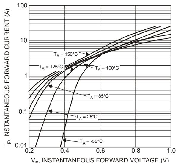
Fig. 2 Typ. Forward Characteristics - B350A thru B360A
