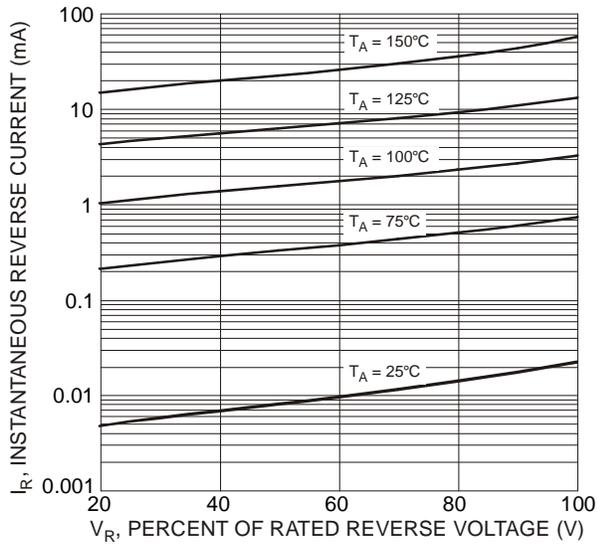
Fig. 3 Typical Reverse Characteristics, B320A thru B340A
