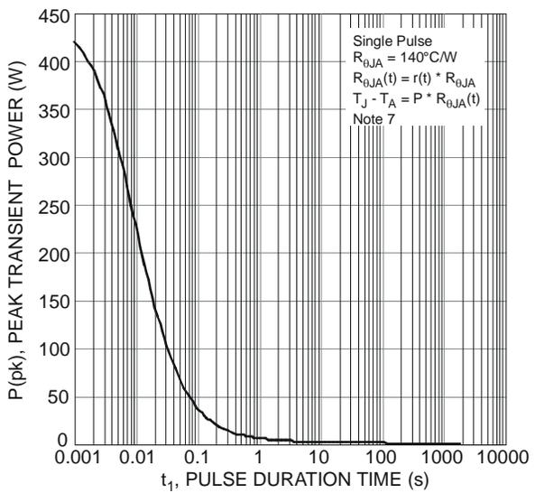
Fig. 11 Single Pulse Maximum Power Dissipation (B320A-B340A)
