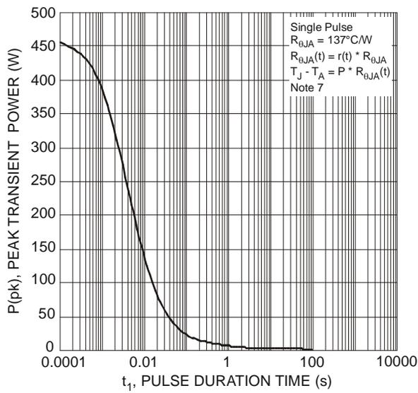
Fig. 12 Single Pulse Maximum Power Dissipation (B350A-B360A)
