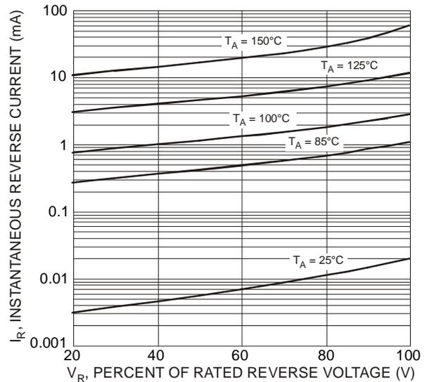
Fig. 4 Typical Reverse Characteristics, B350A thru B360A
