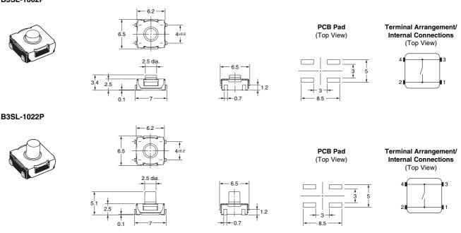
Note: Unless otherwise specified, a tolerance of ±0.2 mm applies to all dimensions.
