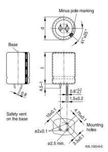
Snap-in terminals, length (6.0  $\pm$ 1) mm. Also available in a shorter version with a length of (4.5 -1) mm.
