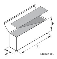
$L \times W \times H$  (max. mm): Axial:  $310 \times 75 \times 120$ , radial:  $340 \times 50 \times 210$
