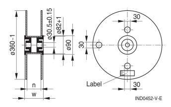
n (mm): Axial 72 +1, radial 42 +1 w (mm): Axial 84 max., radial 54 max.
