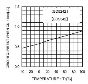
Fig.10 Circuit Current when ON
