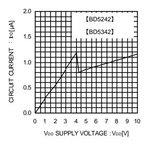
Fig.3 Circuit Current
