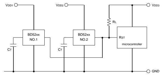
Fig.20 OR Circuit Connection Application
