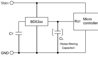
Fig.19 CMOS Output Type
