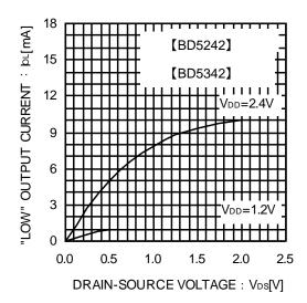
Fig.4 "Low" Output Current
