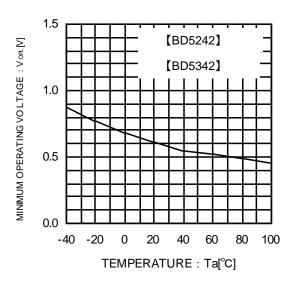
Fig.12 Operating Limit Voltage
