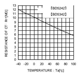
Fig.13 CT Terminal Circuit Resistance
