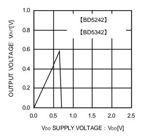
Fig.7 Operating Limit Voltage
