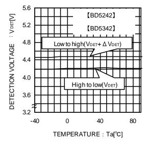
Fig.9 Detection Voltage Release Voltage
