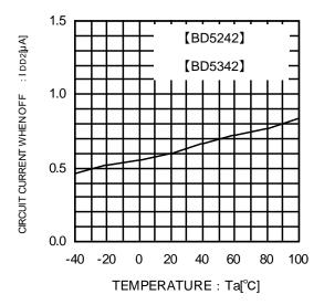
Fig.11 Circuit Current when OFF
