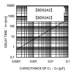
Fig.14 Delay Time (t<sub>PLH</sub>) and C<sub>T</sub> Terminal External Capacitance
