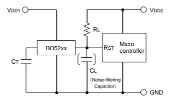
Fig.18 Open Drain Output Type
