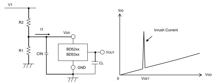
Fig.21 Resistor Divider Connection Application
