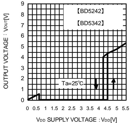
Fig.6 I/O Characteristics
