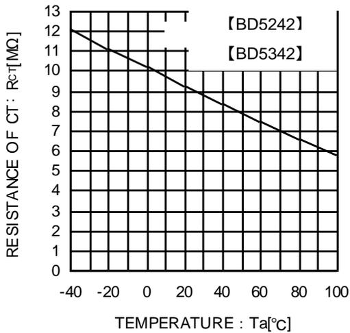
Fig.13 C<sub>T</sub> Terminal Circuit Resistance
