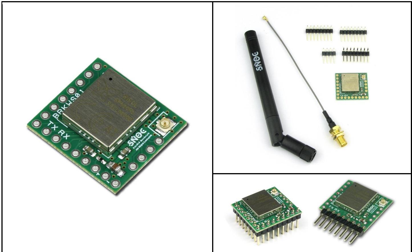
The breakout BRKWS01 is a very small footprint SigFox breakout board based on the Wisol SFM10R3 module. This board will enable you to integrate and use the SigFox LPWan network into your IOT project design, providing simple data transmission feature.
