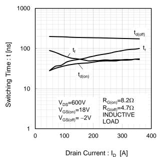
Fig.11 Switching Characteristics [T<sub>i</sub>=150°C]
