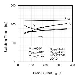
Fig.10 Switching Characteristics [T<sub>i</sub>=125°C]
