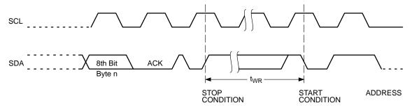
Figure 7. Write Cycle Timing
