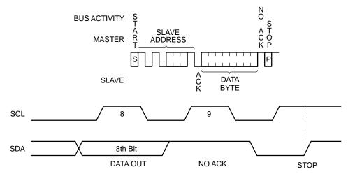
Figure 10. Immediate Read Sequence and Timing
