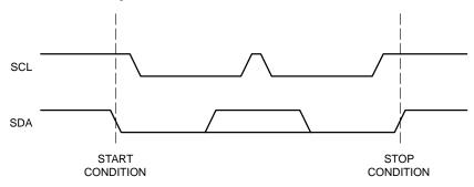
Figure 2. Start/Stop Timing
