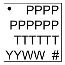
Figure 8.3. QFN20 Package Marking
