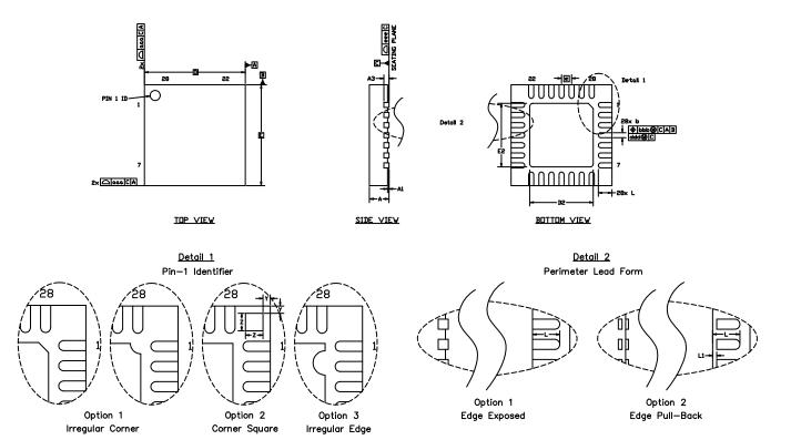
Figure 6.1. QFN28 Package Drawing
