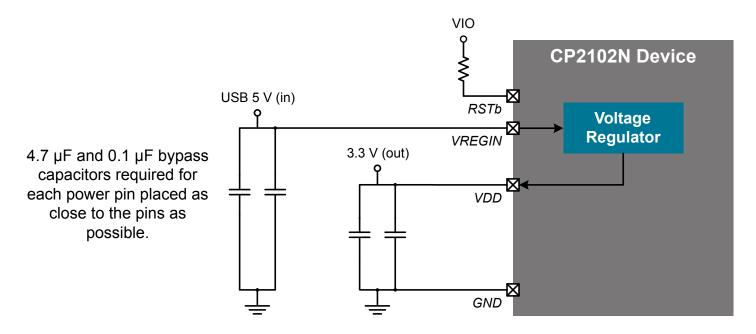
Figure 2.1. Connection Diagram with Voltage Regulator Used and USB Connected (Bus-Powered)
