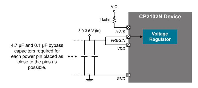
Figure 2.3. Connection Diagram with Voltage Regulator Not Used
