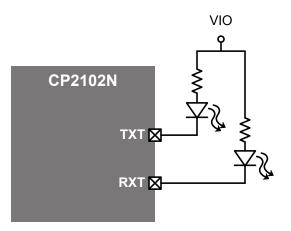
Figure 4.3. Transmit and Receive Toggle
