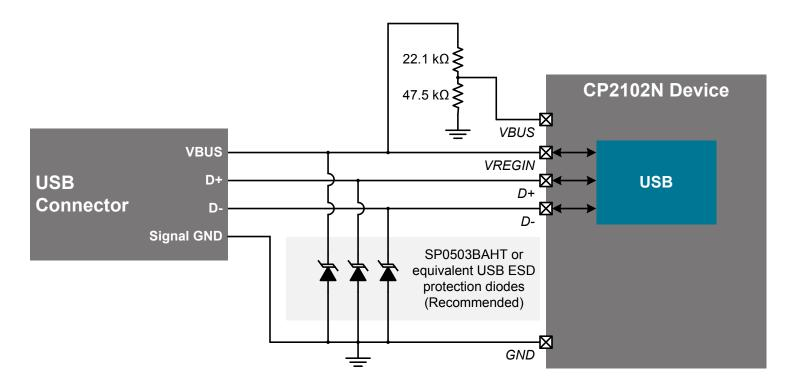
Figure 2.5. Bus-Powered Connection Diagram for USB Pins
