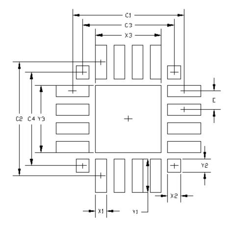
Figure 8.2. QFN20 PCB Land Pattern Drawing
