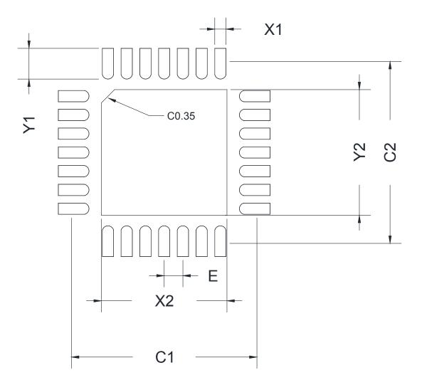
Figure 6.2. QFN28 PCB Land Pattern Drawing
