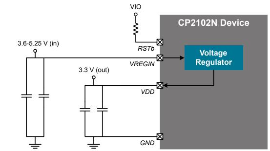
4.7 μF and 0.1 μF bypass capacitors required for each power pin placed as close to the pins as possible.
