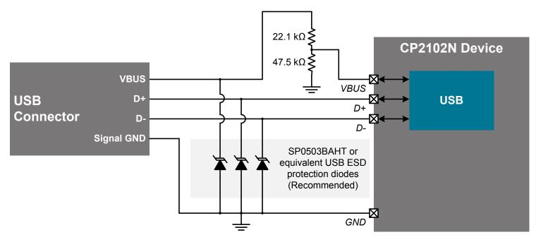
Figure 2.6. Self-Powered Connection Diagram for USB Pins
