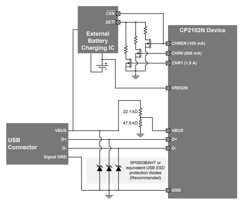
Figure 2.4. Battery Charging Connection Diagram
