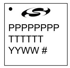
Figure 6.3. QFN28 Package Marking
