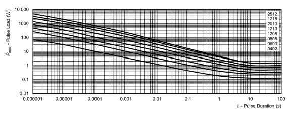
Maximum pulse load, single pulse; applicable if  $\bar{P} \rightarrow 0$  and n < 1000 and  $\hat{U} \le \hat{U}_{max.}$ ; for permissible resistance change equivalent to 8000 h operation
