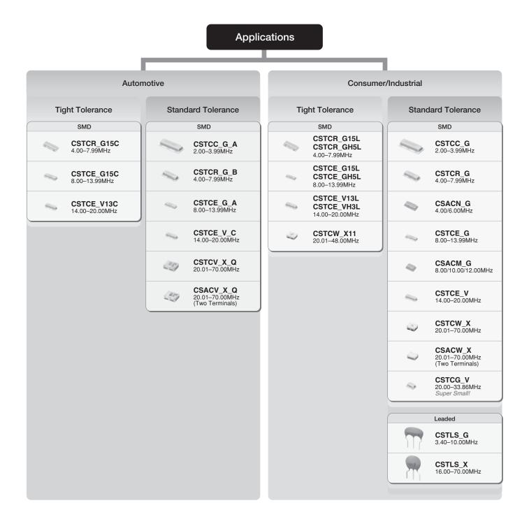
Notice: "CERALOCK<sup>®</sup> for consumer" and "CERALOCK<sup>®</sup> for automotive" is different in the specification of Operating Temperature Range, Environmental Characteristics, Physical Characteristics and so on. Please choose either "for consumer" or "for automotive" according to the required specification.
