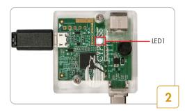
Connect the CY4500 EZ-PD™ Protocol Analyzer to your PC via the USB2.0 Type-A to Micro-B Cable provided with the Analyzer. Observe LED1 (white color) blink continuously
