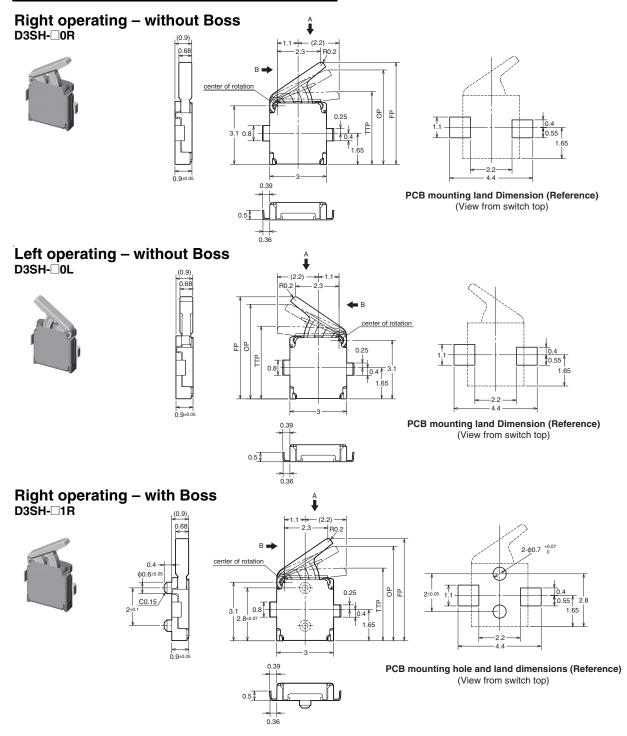
Note: 1. Unless otherwise specified, all units are in millimeters and a tolerance of ±0.15 mm applies to all dimensions
