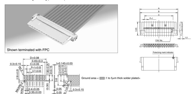
Signal area <  $\boxtimes\boxtimes$ :1 to 5 $\mu$ m thick solder plated>
