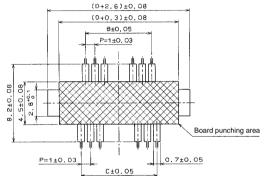
Note: The 2.9mm board to board size does not include the soldering paste thickness.
