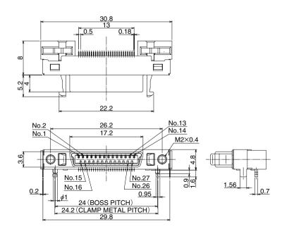
The product information in this catalog is for reference only. Please request the Engineering Drawing for the most current and accurate design information. DH Series•High speed transmission, 1mm pitch Small Interface Connector
