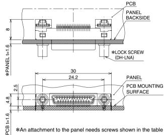
\*An attachment to the panel needs screws shown in the table below.
