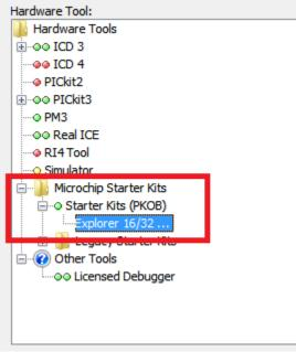
If the device does not appear within the Hardware Tool list, make sure that the selected target microcontroller in the project exactly matches the part number of the microcontroller on the PIM, and that the PKOB supports the target selected, as indicated by a green or yellow circular icon next to the "Starter Kits (PKOB)" line in the Hardware Tool menu.
