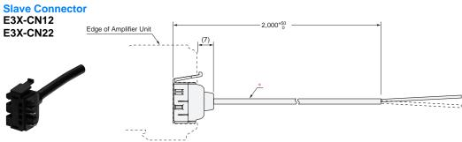
\* E3X-CN12: 2.6-dia. cable with 1 conductor, Standard cable length: 2 m (Conductor cross-section: 0.2 mm² (AWG24), Insulator diameter: 1.1 mm) E3X-CN22: 4-dia. cable with 2 conductors, Standard cable length: 2 m (Conductor cross-section: 0.2 mm² (AWG24), Insulator diameter: 1.1 mm)
