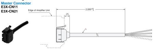
\* E3X-CN11: 4-dia. cable with 3 conductors, Standard cable length: 2 m (Conductor cross-section: 0.2 mm² (AWG24), Insulator diameter: 1.1 mm) E3X-CN21: 4-dia. cable with 4 conductors, Standard cable length: 2 m (Conductor cross-section: 0.2 mm² (AWG24), Insulator diameter: 1.1 mm)
