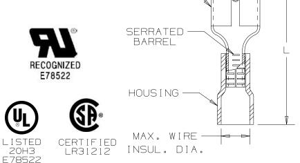
VINYL INSULATED, BUTTED SEAM #22-14 AWG CUSTOMER DRAWING ITEM REVISION NAME 00123SHJ/00 DATASET FILE NAME 00123SHJ/00 MATERIAL:
