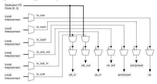
Figure 2-24. Control Signal Selection per IOE
