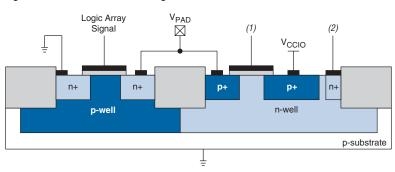
Figure 4–2. Transistor Level Diagram of FPGA Device I/O Buffers
