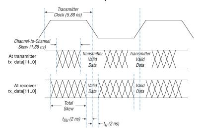
Figure 5-5. RSDS Transmitter Clock to Data Relationship
