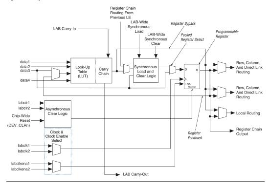
Each LE's programmable register can be configured for D, T, JK, or SR operation. Each register has data, clock, clock enable, and clear inputs. Signals that use the global clock network, general-purpose I/O pins, or any internal logic can drive the register's clock and clear control signals. Either general-purpose I/O pins or internal logic can drive the clock enable. For combinational functions, the LUT output bypasses the register and drives directly to the LE outputs.
