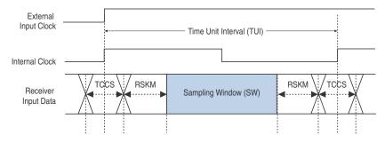
Figure 5–4 shows the high-speed I/O timing budget.
