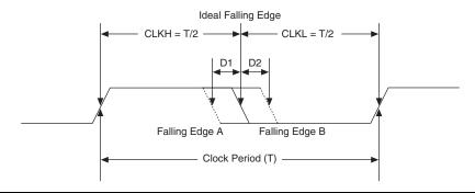
DCD expressed in absolution derivation, for example, D1 or D2 in Figure 5–8, is clock-period independent. DCD can also be expressed as a percentage, and the percentage number is clock-period dependent. DCD as a percentage is defined as:
