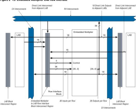
Figure 2-19. Embedded Multiplier LAB Row Interface
