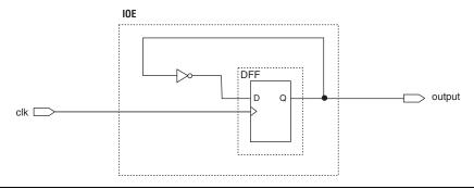
However, when the output is a double data rate input/output (DDIO) signal, both edges of the input clock signal (positive and negative) trigger output transitions (Figure 5–10). Therefore, any distortion on the input clock and the input clock buffer affect the output DCD.
