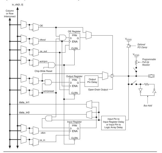
Figure 2–25. Cyclone II IOE in Bidirectional I/O Configuration
