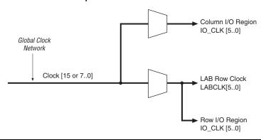
LAB row clocks can feed LEs, M4K memory blocks, and embedded multipliers. The LAB row clocks also extend to the row I/O clock regions.
