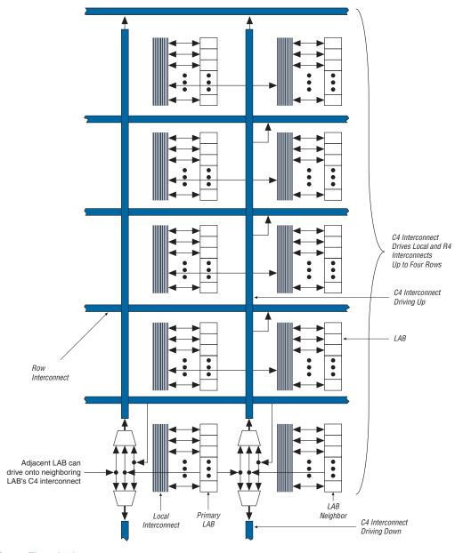
Figure 2–10. C4 Interconnect Connections Note (1)
