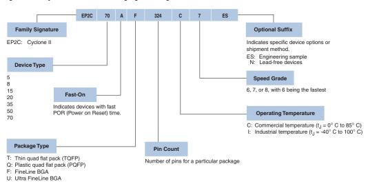
Figure 6-1. Cyclone II Device Packaging Ordering Information
