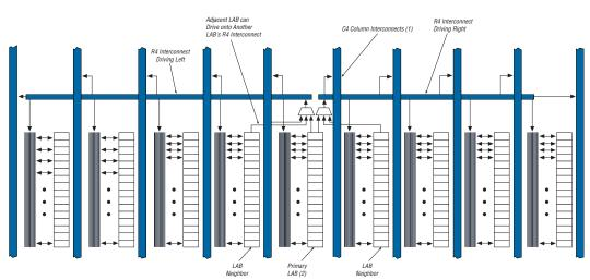
Figure 2-8. R4 Interconnect Connections
