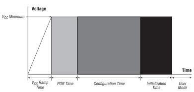
Figure 4-3. Cyclone II Wake-Up Time
