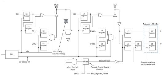
Figure 2-27. DDR SDRAM Interfacing
