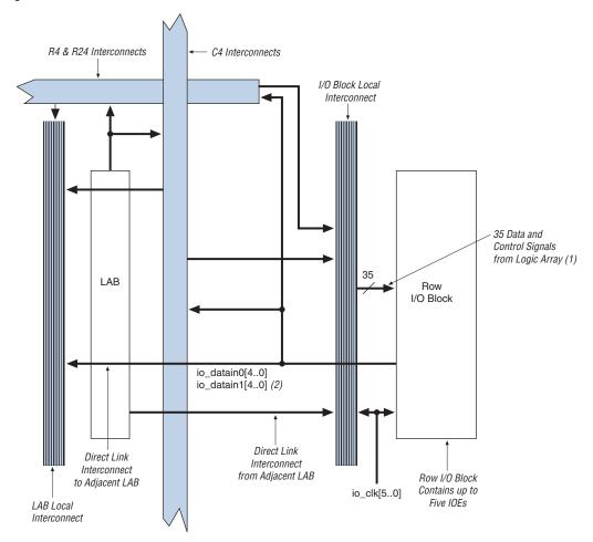
Figure 2-21. Row I/O Block Connection to the Interconnect
