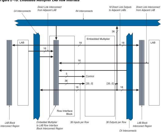
Figure 2-19. Embedded Multiplier LAB Row Interface
