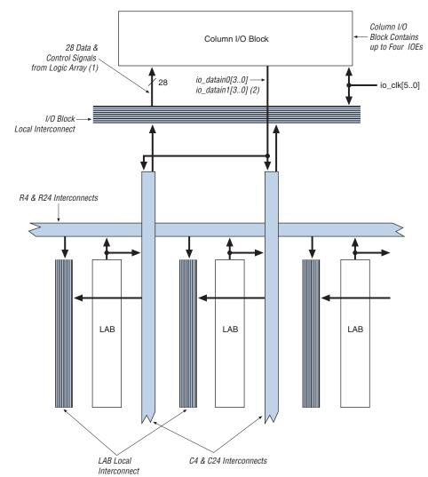
Figure 2-22. Column I/O Block Connection to the Interconnect
