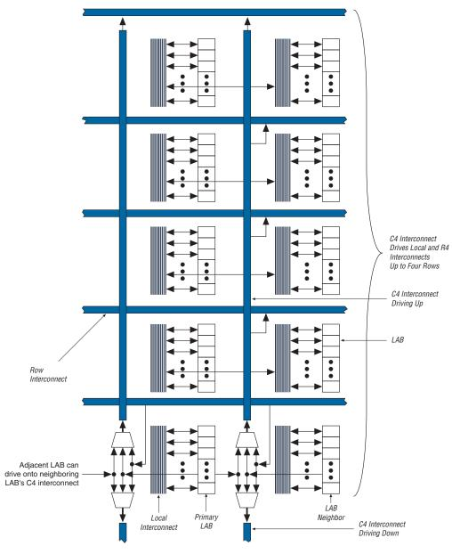
Figure 2–10. C4 Interconnect Connections Note (1)
