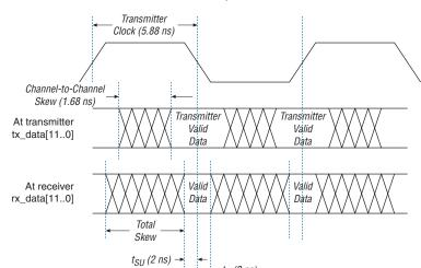
Figure 5-5. RSDS Transmitter Clock to Data Relationship
