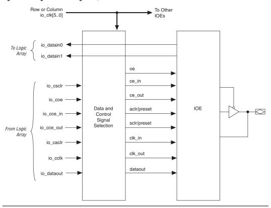
Figure 2-23. Signal Path Through the I/O Block
