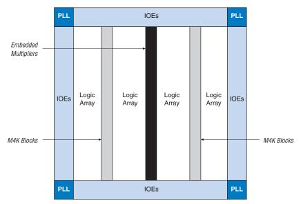
Figure 2–1. Cyclone II EP2C20 Device Block Diagram
