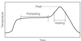
For soldering (Example: Sn/Pb)
