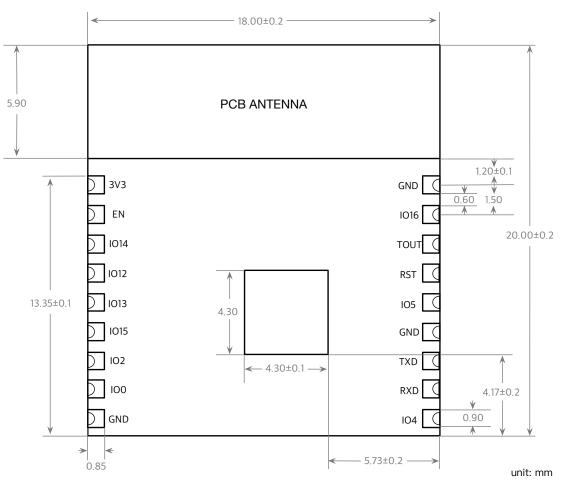
Figure 2-1 shows the pin distribution of the ESP-WROOM-02.
