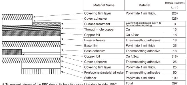
\* To prevent release of the FPC due to its bending, use of the double sided FPC with copper foil on the back side is NOT RECOMMENDED.
