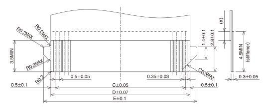
Note 1 : Stiffener dimension should be 3.5mm min., and X dimension should be 0.5mm for improved flexibility of FPC.
