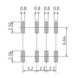
• PC board mounting pad layout (TOP VIEW)
