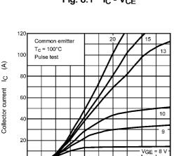
Collector-emitter voltage  $V_{CE}$  (V) Fig. 8.3 I<sub>C</sub> -  $V_{CE}$
