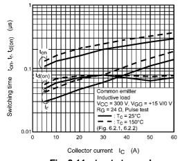
Fig. 8.11  $t_{on}$ ,  $t_{r}$ ,  $t_{d(on)}$  -  $I_{C}$
