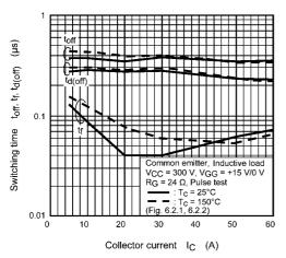
Fig. 8.13  $t_{off}$ ,  $t_f$ ,  $t_{d(off)-IC}$
