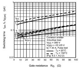
Fig. 8.10  $t_{on}$ ,  $t_r$ ,  $t_{d(on)}$  -  $R_G$
