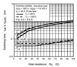
Fig. 8.12 t<sub>off</sub>, t<sub>f</sub>, t<sub>d(off)</sub> - R<sub>G</sub>
