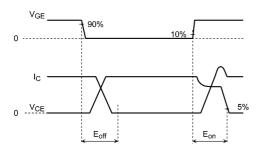
Fig. 6.2.3 Timing Chart of Switching Loss
