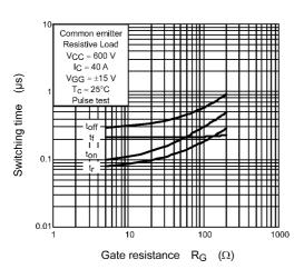
Fig. 8.9 Switching Time - R<sub>G</sub>
