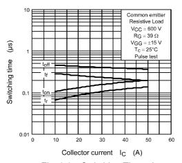
Fig. 8.8 Switching Time - I<sub>C</sub>
