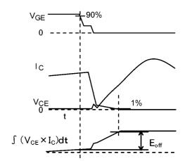
Fig. 6.2.4 Timing Chart of Switching Loss
