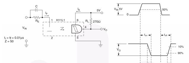
Figure 7. Switching Test Circuit and Waveforms
