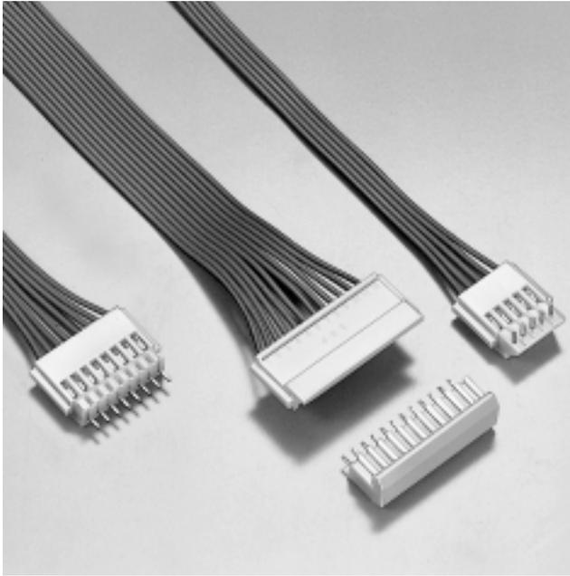
**This 2.5mm (.098") pitch connector is used to connect wires to printed circuit boards. The header is available in three configurations : top, side, and bottom entry. This allows the wires to be perpendicular or parallel to the printed circuit board in any direction.**
