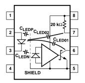
Figure 17. Optocoupler input to output capacitance model for shielded optocouplers.
