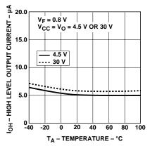
Figure 3. High level output current vs. temperature.
