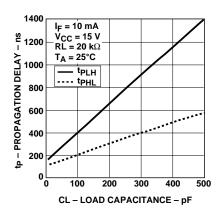
Figure 11. Propagation delay vs. load
