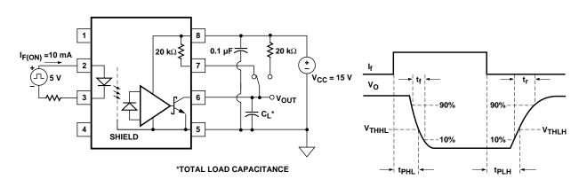
Figure 6. Propagation delay test circuit.
