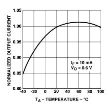
Figure 2. Normalized output current vs. temperature.
