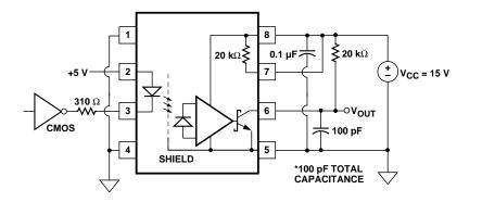
Figure 15. Recommended LED drive circuit.
