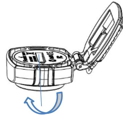
④ Screw clockwise the battery cover tight with a coin or the headlamp buckle.
