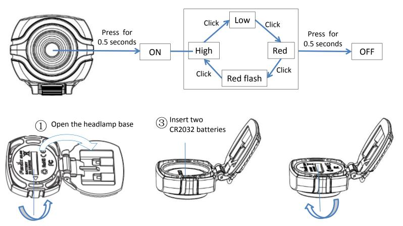
② Use headlamp buckle or one coin to insert the battery cover slot, contrarotate about 45 degree to open the battery cover.
