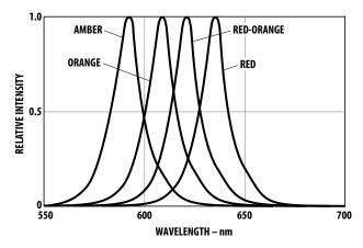
Figure 1. Relative intensity vs. peak wavelength
