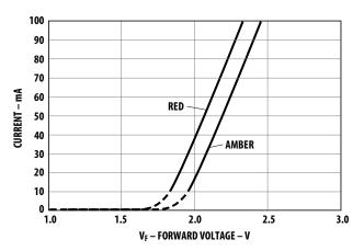
Figure 2. Forward current vs. forward voltage
