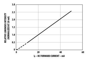
Figure 3. Relative luminous intensity vs. forward current
