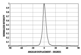
Figure 5. Representative spatial radiation pattern for  $8^{\circ}$  viewing angle lamps
