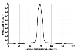
Figure 6. Representative spatial radiation pattern for 15° viewing angle lamps
