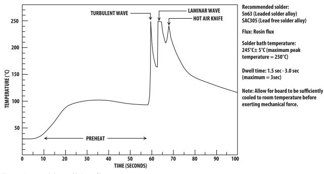
Figure 10. Recommended wave soldering profile
