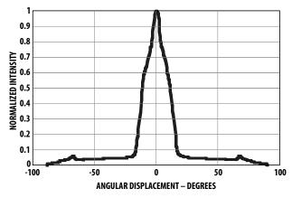
Figure 7. Representative spatial radiation pattern for 23  $^{\circ}$  viewing angle lamps
