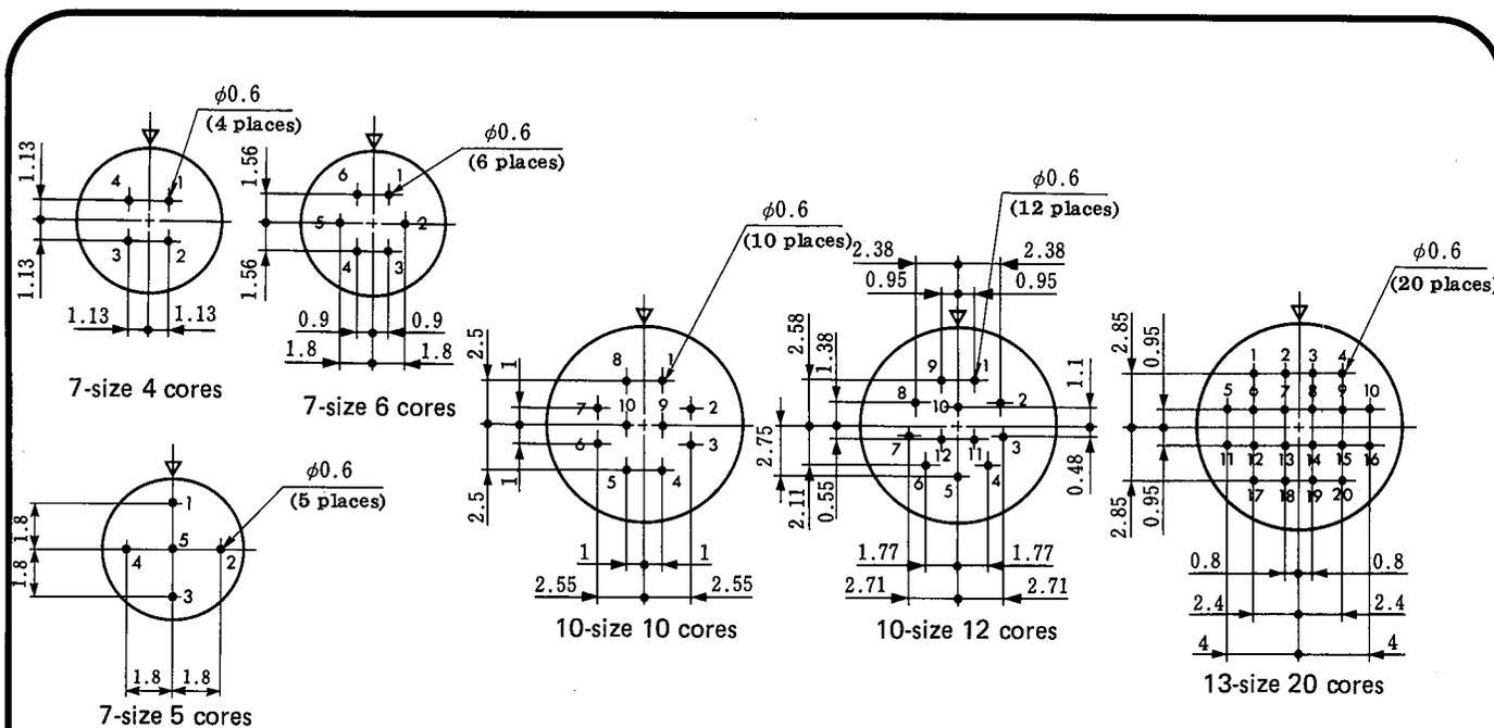
Remarks: 1. The above figures are views of receptacle-socket inserts from the mating side and plug-pin inserts from the wiring-connection side.
