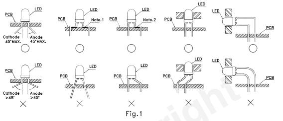
) " Correct mounting method "imes" Incorrect mounting method
