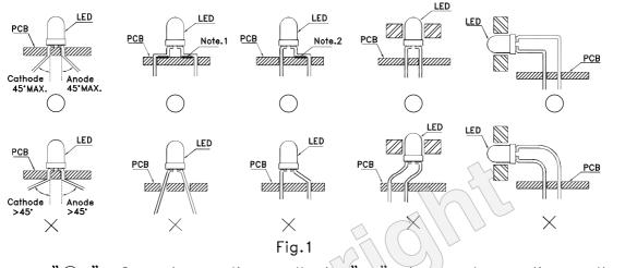
" $\bigcirc$ " Correct mounting method " $\times$ " Incorrect mounting method
