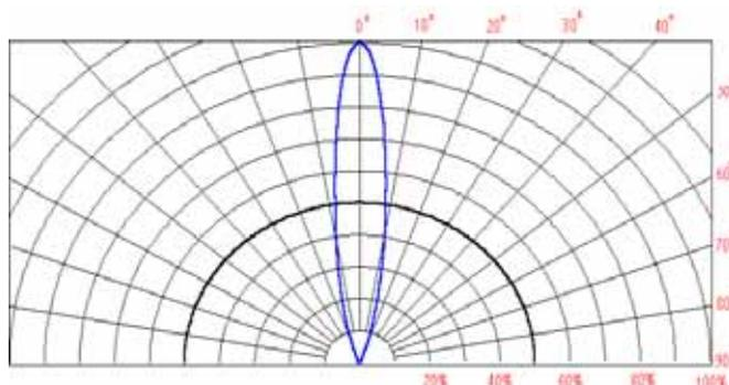
\* Duty 1/10 Pulse Width 0.1ms At the position of 4mm from the bottom of the package
