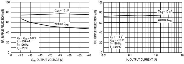
Figure 11. Ripple Rejection versus Output Voltage
