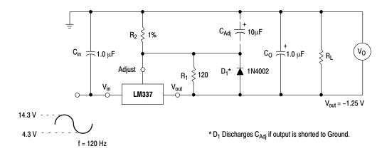
Figure 4. Ripple Rejection Test Circuit
