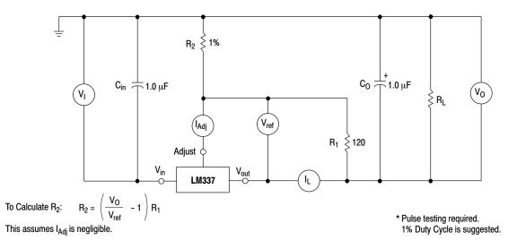
Figure 3. Standard Test Circuit
