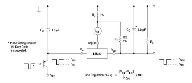
Figure 1. Line Regulation and  $\Delta I_{\text{Adj}}/\text{Line Test Circuit}$
