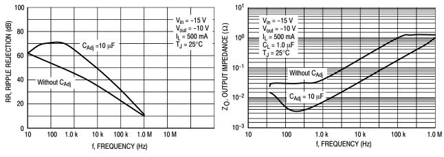
Figure 13. Ripple Rejection versus Frequency
