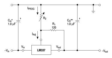
$^*C_{in}$  is required if regulator is located more than 4 inches from power supply filter. A 1.0  $\mu F$  solid tantalum or 10  $\mu F$  aluminum electrolytic is recommended.
