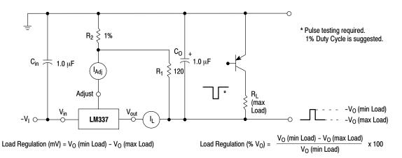
Figure 2. Load Regulation and  ${\bigtriangleup I}_{\text{Adj}}\text{/}\text{Load}$  Test Circuit
