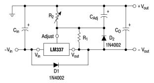
Figure 18. Voltage Regulator with Protection Diodes
