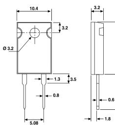
Mechanical Protection Resistive Element Substrate Connections Weight Mounting Torqure Molded Thick film Alumina Tinned copper 2 g max. 1 Nm
