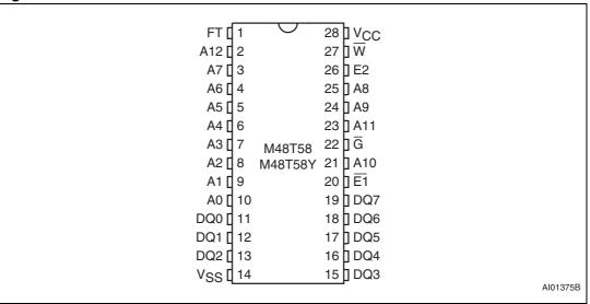
Figure 3. SOIC connections
