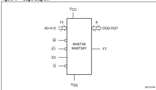
Figure 1. Logic diagram
