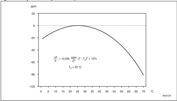
Figure 9. Clock calibration
