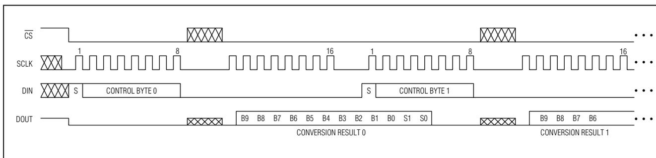
Figure 11b. External Clock Mode, 16 Clocks/Conversion Timing
