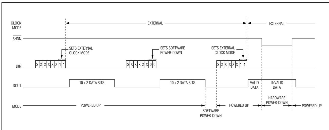
Figure 12a. Timing Diagram Power-Down Modes, External Clock
