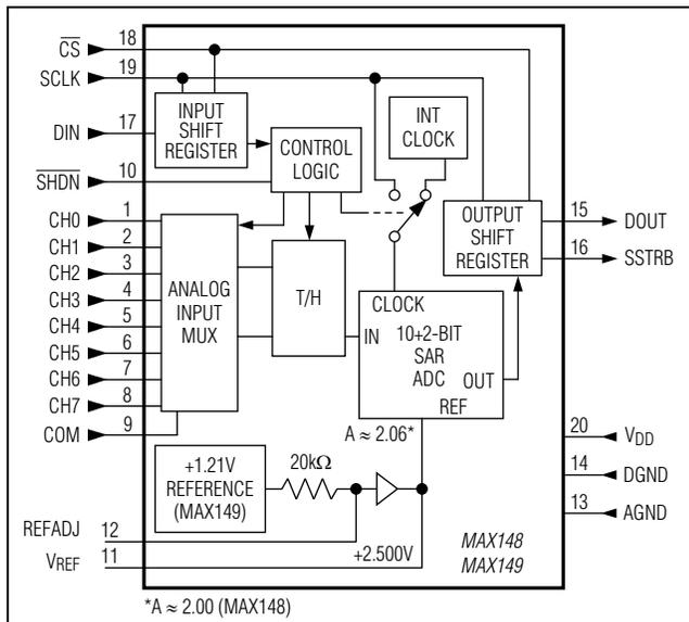
Figure 3. Block Diagram
