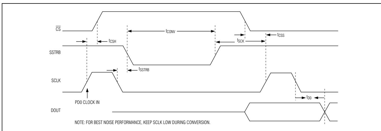
Figure 10. Internal Clock Mode SSTRB Detailed Timing
