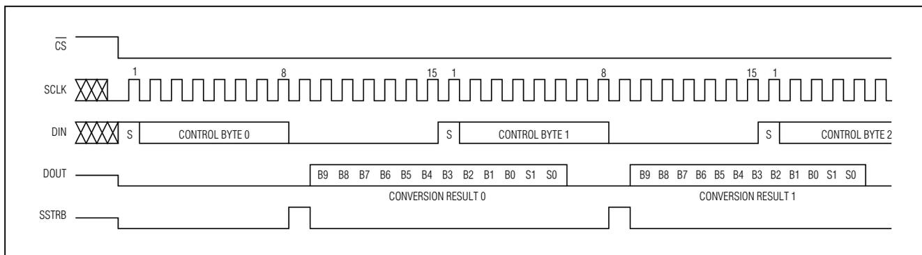
Figure 11a. External Clock Mode, 15 Clocks/Conversion Timing
