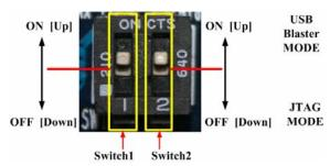
Figure 2.10. Set both switches to UP position to set up the MAX II Micro board as a USB Blaster.
