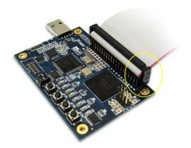
Figure 4.6. The connection setup for the 40-pin cable with MAX II Micro board.
