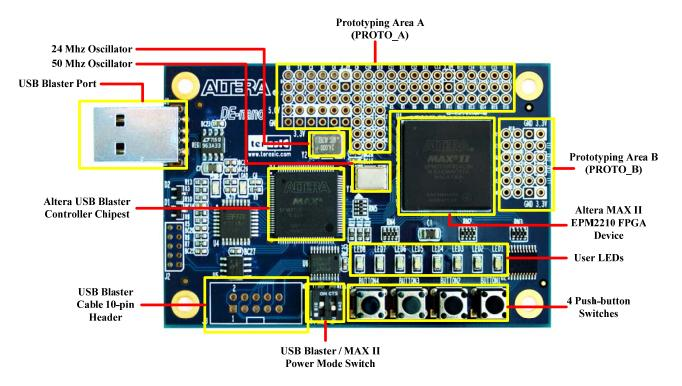
Figure 2.1. The MAX II Micro board.
