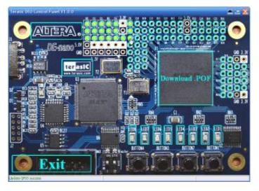
Figure 3.6 Users can configure the GPIOs in the prototyping areas by clicking on the corresponding holes shown in the Control Panel window section. The GPIOs' color will be marked by yellow to indicate their voltage level is HIGH (3.3V).
