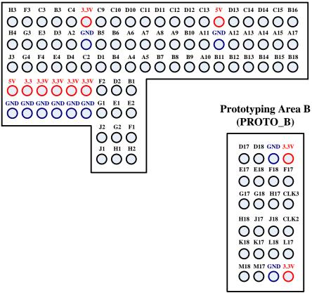
Figure 2.7. The detailed I/O map of prototyping area A and B.
