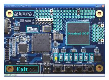
Figure 3.4 Control panel window for LED controlling.
