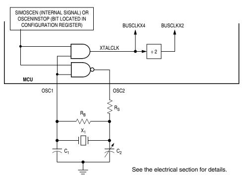
Figure 11-2. XTAL Oscillator External Connections
