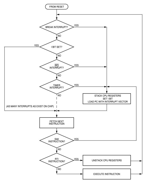
Figure 13-7. Interrupt Processing
