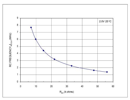
Figure 16-12. RC versus Frequency (2 Volts @ 25°C)
