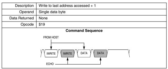
A sequence of IREAD or IWRITE commands can access a block of memory sequentially over the full 64-Kbyte memory map.
