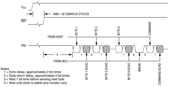
Figure 15-16. Monitor Mode Entry Timing
