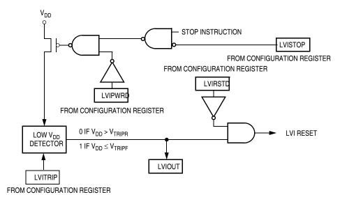
Figure 10-1. LVI Module Block Diagram
