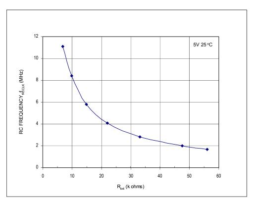
Figure 16-10. RC versus Frequency (5 Volts @ 25°C)
