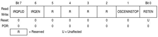
Figure 5-1. Configuration Register 2 (CONFIG2)
