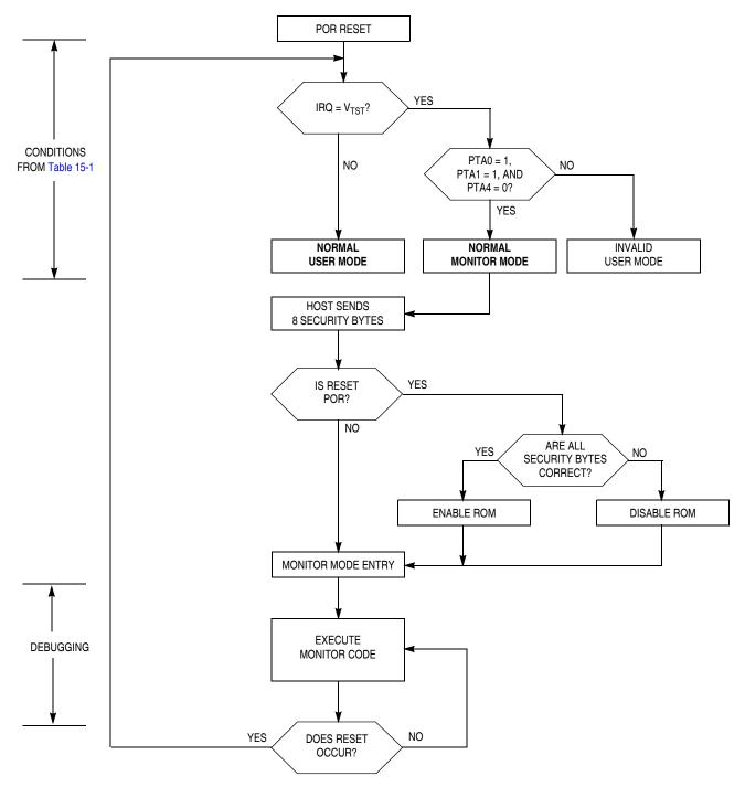
Figure 15-9. Simplified Monitor Mode Entry Flowchart
