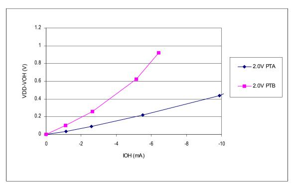
Figure 16-7. Typical 2-Volt Output High Voltage versus Output High Current (25°C)
