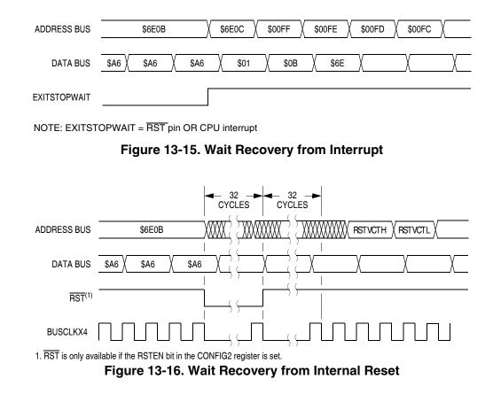
Figure 13-15 and Figure 13-16 show the timing for wait recovery.
