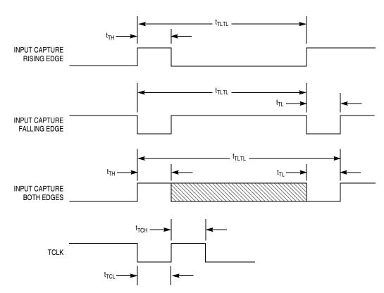
Figure 16-16. Timer Input Timing
