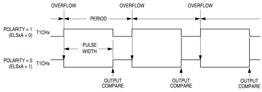
Figure 14-3. PWM Period and Pulse Width
