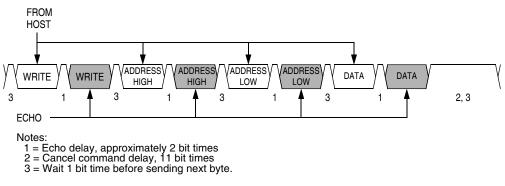
Figure 15-14. Write Transaction
