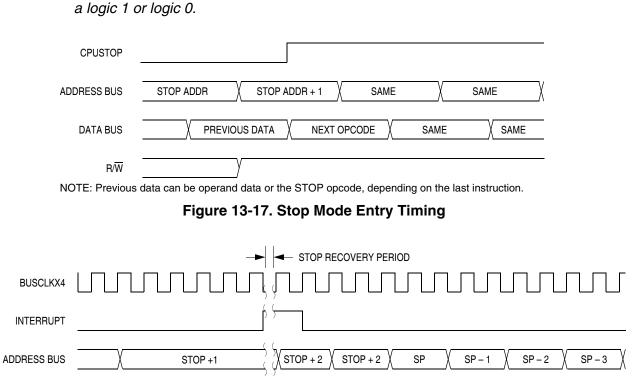
Figure 13-18. Stop Mode Recovery from Interrupt
