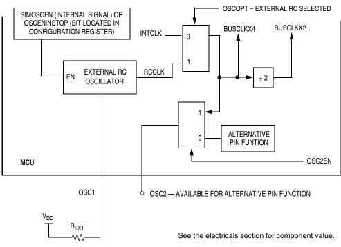
Figure 11-3. RC Oscillator External Connections
