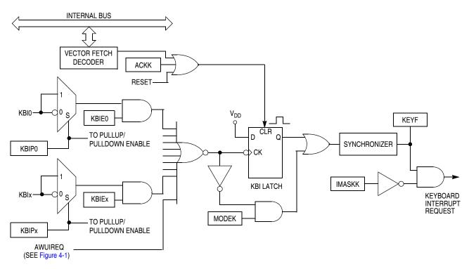
Figure 9-2. Keyboard Interrupt Block Diagram
