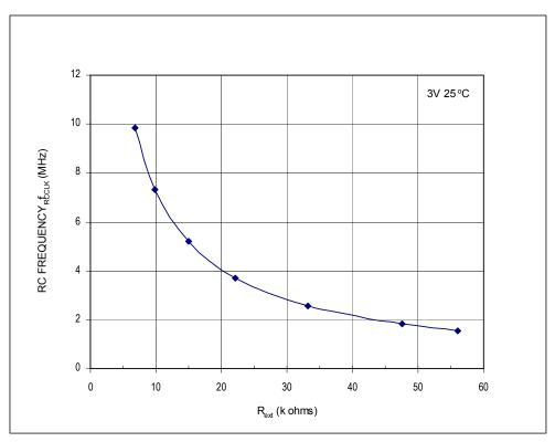
Figure 16-11. RC versus Frequency (3 Volts @ 25°C)
