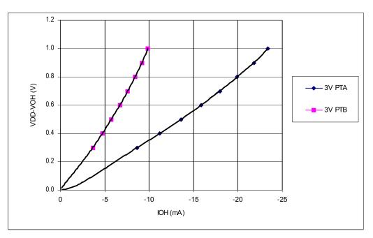
Figure 16-4. Typical 3-Volt Output High Voltage versus Output High Current (25°C)
