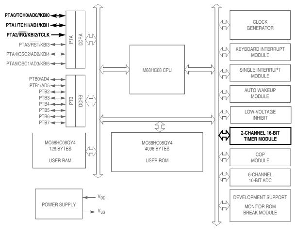
RST, IRQ: Pins have internal pull up device All port pins have programmable pull up device PTA[0:5]: Higher current sink and source capability PTB[0:7]: Not available on 8-pin devices
