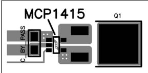
FIGURE 4-3: Recommended PCB Layout (TOP).
