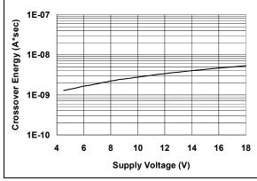
FIGURE 2-21: Crossover Energy vs. Supply Voltage.
