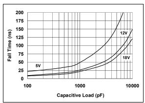
FIGURE 2-5: Fall Time vs. Capacitive Load.
