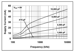
FIGURE 2-18: Supply Current vs. Frequency.
