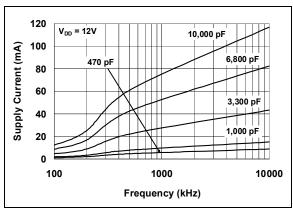
**FIGURE 2-17:** Supply Current vs. Frequency.
