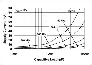
FIGURE 2-14: Supply Current vs. Capacitive Load.
