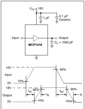
FIGURE 4-2: Non-Inverting Driver Timing Waveform.
