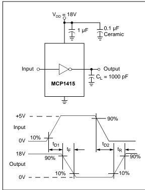
FIGURE 4-1: Inverting Driver Timing Waveform.
