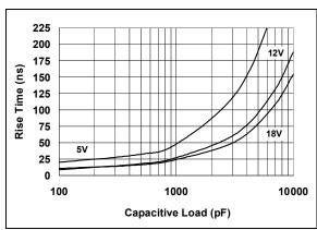
**FIGURE 2-2:** Rise Time vs. Capacitive Load.
