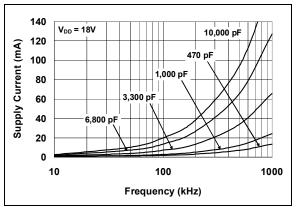
**FIGURE 2-16:** Supply Current vs. Frequency.
