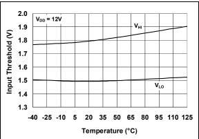
FIGURE 2-12: Input Threshold vs. Temperature.
