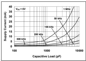
FIGURE 2-15: Supply Current vs. Capacitive Load.
