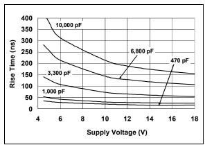
**FIGURE 2-1:** Rise Time vs. Supply Voltage.
