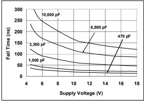
**FIGURE 2-4:** Fall Time vs. Supply Voltage.
