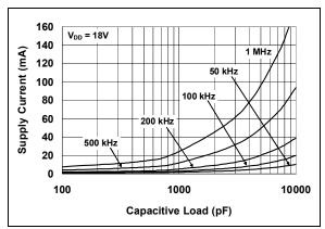
FIGURE 2-13: Supply Current vs. Capacitive Load.
