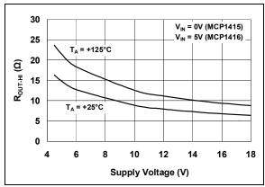
**FIGURE 2-19:** Output Resistance (Output High) vs. Supply Voltage.
