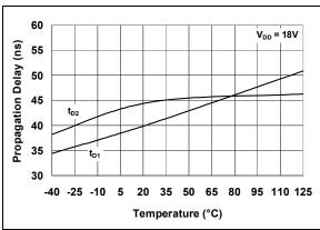
**FIGURE 2-8:** Propagation Delay Time vs. Temperature.
