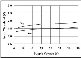
FIGURE 2-11: Input Threshold vs. Supply Voltage.
