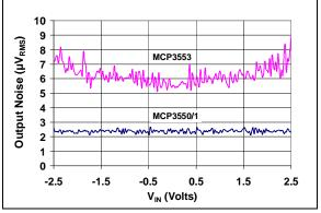
**FIGURE 2-6:** Output Noise vs. Input Voltage ( $V_{DD} = 2.7V$ ).
