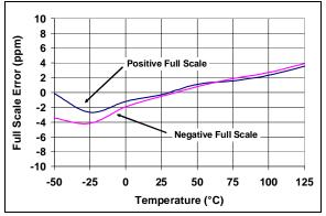
FIGURE 2-14: Full Scale Error vs. Temperature.
