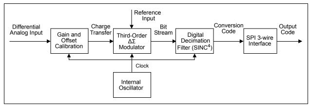
FIGURE 4-1: MCP3550/1/3 Functional Block Diagram.
