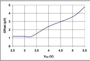
FIGURE 2-11: Offset Error vs VDD  $(V_{CM} = 0V).$
