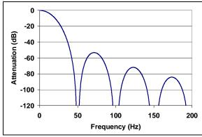
FIGURE 4-2: SINC Filter Response, MCP3550-50 Device.
