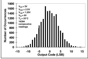
FIGURE 2-17: MCP3553 Output Noise Histogram.
