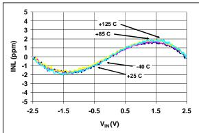
FIGURE 2-1:INL Error vs. Input Voltage(V<sub>DD</sub> = 2.7V).
