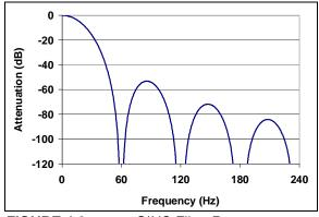
FIGURE 4-3: SINC Filter Response, MCP3550-60 Device.
