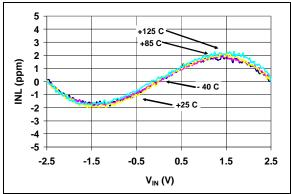
FIGURE 2-2: INL Error vs. Input Voltage  $(V_{DD} = 5.0V)$ .
