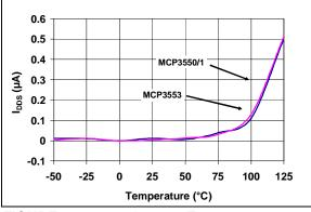
FIGURE 2-24: I<sub>DDS</sub> vs. Temperature.
