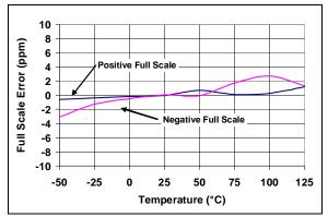
**FIGURE 2-15:** Full Scale Error vs. Temperature ( $V_{REF} = 5.0V$ ).
