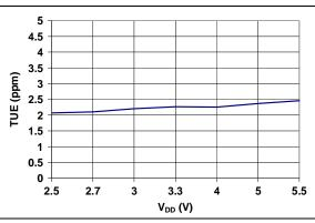
FIGURE 2-23: Maximum TUE vs. V<sub>DD</sub>.
