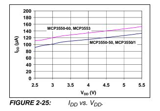
**Note:** Unless otherwise specified,  $T_A = +25^{\circ}C$ ,  $V_{DD} = 5V$ ,  $V_{REF} = 2.5V$ ,  $V_{SS} = 0V$ ,  $V_{CM} = V_{REF}/2$ ,  $V_{IN} + = V_{IN}$ . All ppm units use 2\* $V_{REF}$  as full scale range. Unless otherwise noted, graphs apply to entire MCP3550/1/3 family.
