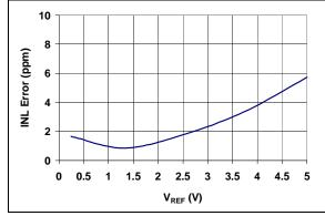
FIGURE 2-4: Maximum INL Error vs. V<sub>REF</sub>.
