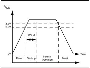
FIGURE 4-6: Power-On Reset Operation.
