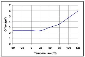
FIGURE 2-12: Offset Error vs. Temperature ( $V_{REF} = 5.0V$ ).
