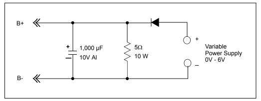
FIGURE 2-2: Simulated Battery Load.
