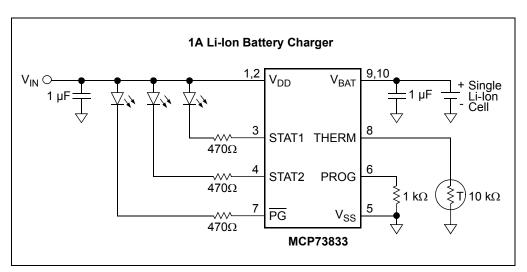
FIGURE 1-1: Typical MCP73833 Application.
